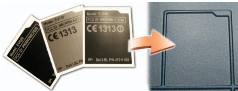
Replace the communications door or the keyboard and affix the regulatory label that matches the color of the bottom of the computer in the space provided.
